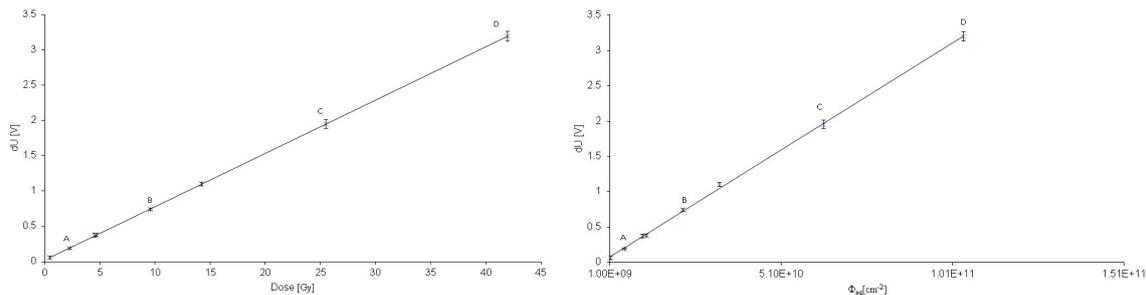
**Figure 1.** S2 PIN diode calibration curve for protons 23 GeV/c dose in Gray (left side) and in NIEL (right side).
