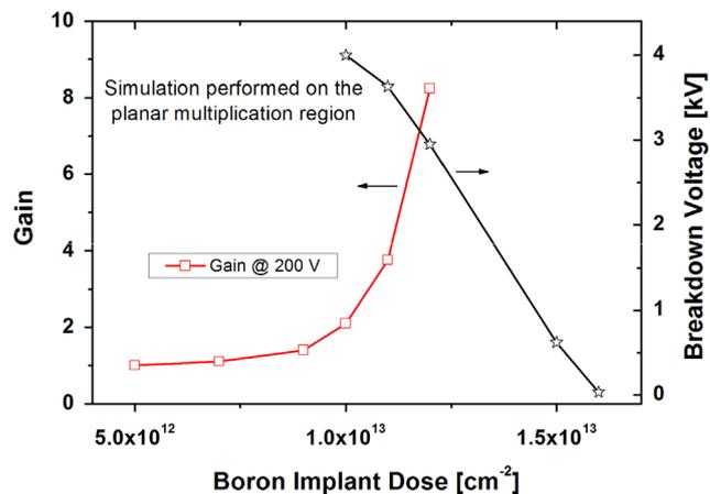
Fig. 2. Simulated dependence of gain and breakdown voltage as a function of the boron dose implanted to form the p well.
