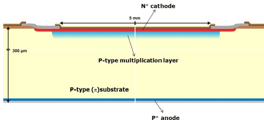
Fig. 1. Schematic cross-section of the LGAD pad design. A p-type layer is diffused below the n+ electrode to form the n+/p/p<sup>-</sup> junction where the multiplication takes place.
