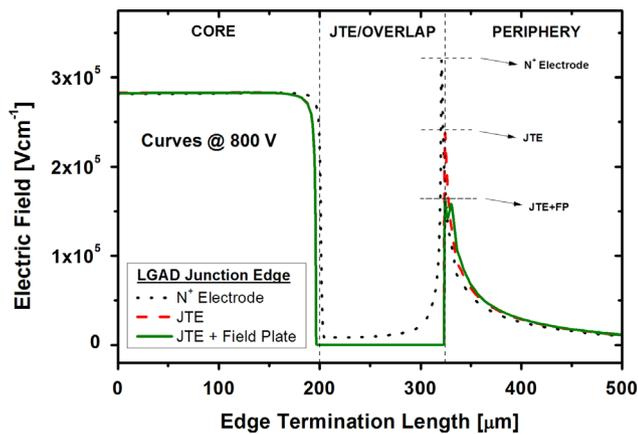
Fig. 3. Simulated electric field distribution at the multiplication junction edge for different termination designs: n<sup>+</sup> electrode extension, JTE, and JTE with field plate.
