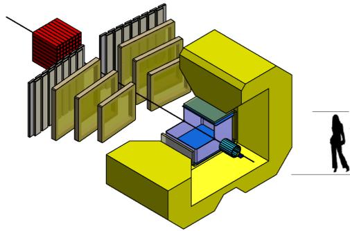
Design of CEE (detector) for fixed target collision at HIAF
