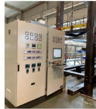
Large size baking furnace commissioning
