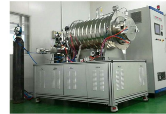
New furnaces for N-doping and infusion study
