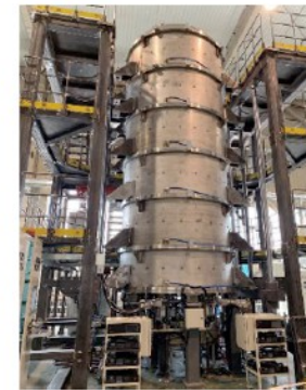
Large size baking furnace commissioning
