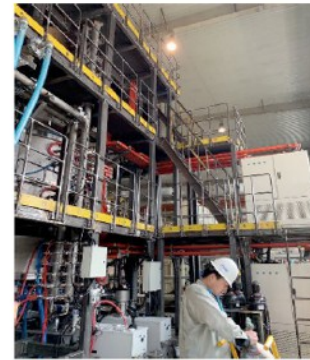
Large size baking furnace commissioning
