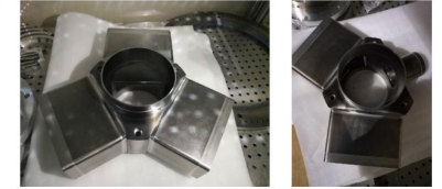
650 MHz 5-cell cavity with waveguide HOM coupler
