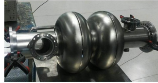
650 MHz 2-cell cavity
