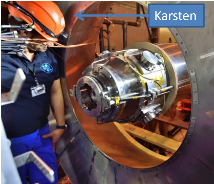
Trouble!! A number of contact fingers are out of place.
