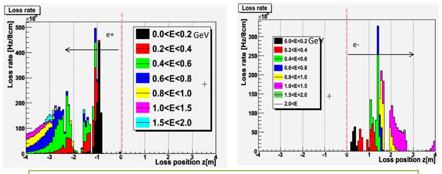
If  $\Delta E$  is large and e+/e- energy becomes less than 2GeV, they can be lost inside the detector (<4m from IP), due to <u>kick by the 1.5T detector solenoid</u> with <u>large crossing angle(41.5mrad)</u>
