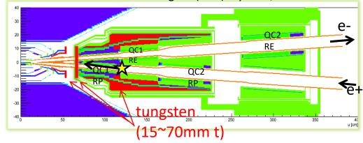
Final focus magnet (QCS) cryostat, R-side
