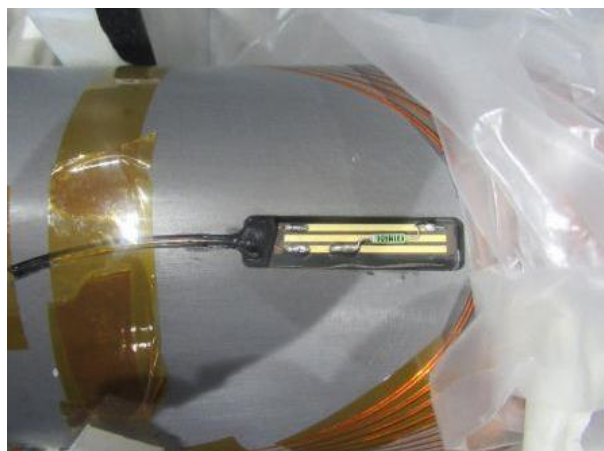
Fabrication of the 2.2m prototype CCT Magnet
