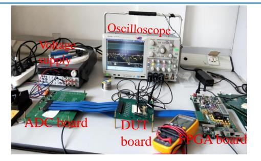
**Current test system for SUPIX-1**
