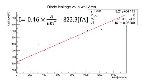
The area of p-well has much effect on the diode capacitance and leakage, and roughly increase linearly against the p-well area. But it has little impact on the charge collection. In order to keep the sensor noise low, the area of the p-well should be as small as possible. For SUPIX-2,  $60 \times 60 \ \mu m^2$  pixel size and 140  $\ \mu m^2$  p-well have been chosen considering the circuit design.
