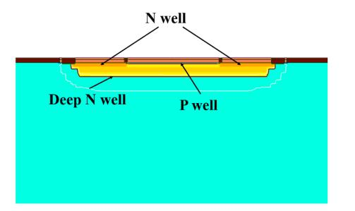
Side view of a pixel sensor
