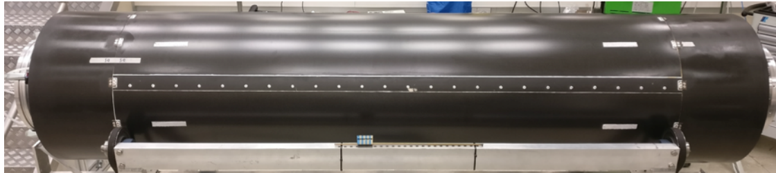
mounting end-plates extensions wrapping in controlled atmosphere
