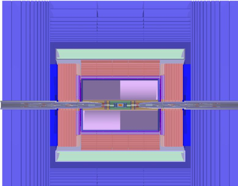
**Baseline detector:** pixel vertex detector, silicon inner tracker, a TPC, Si external tracker, ECAL, HCAL, 3 T B-field, embedded muon detector
