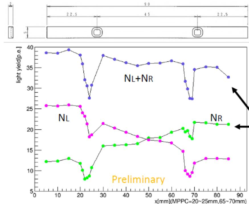
Dimple shape is not same with ECAL prototype
