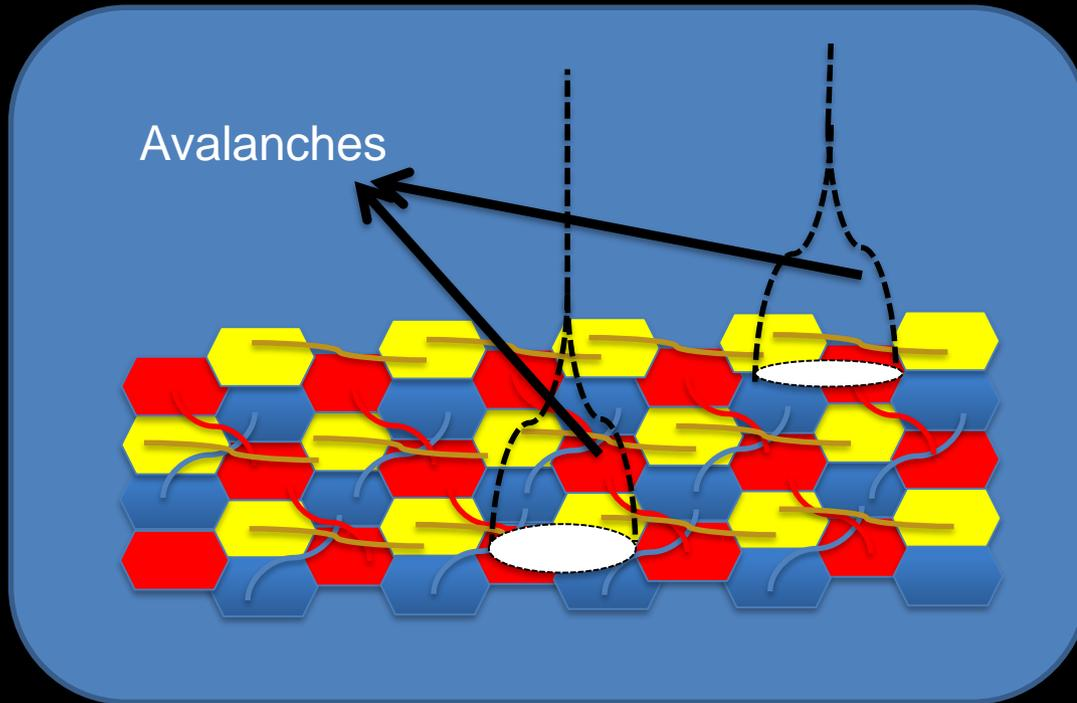
The principle is simple: the **charge is shared among several pads/pixels**. The **pads/pixels are inter-connected in a smart way** so one can identify the position of the impinging particle by identifying the fired strips and thus find the hit as the crossing points.
