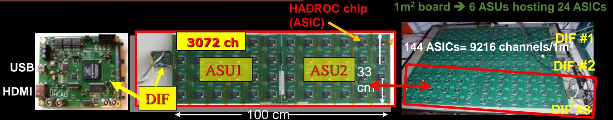
1 DIF (detector InterFace) for 2 ASU (Active Sensor Unit.- PCB+ASICs)
