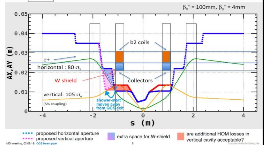
Beam loss inside QC1 can be moved upstream by squeezing upstream beam pipe?
