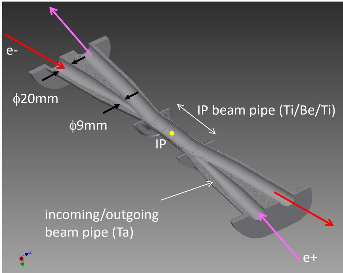
Inner surface of Be pipe is coated with Au layer (10um)
