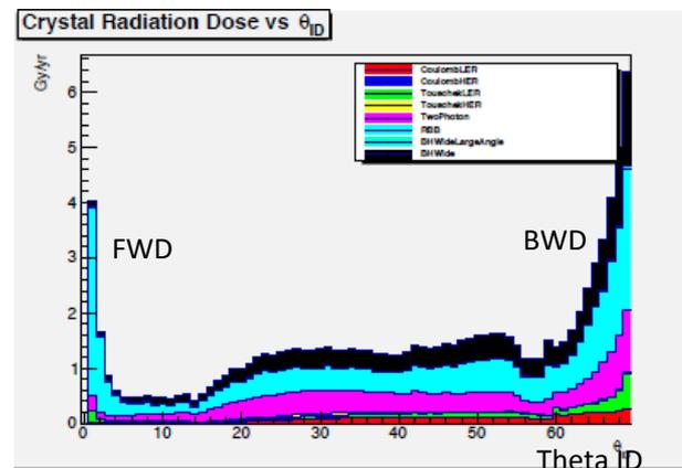
Simulation shows that sub-detectors will survive ~10 years at full luminosity (except TOP PMTs, which will be replaced in few years)
