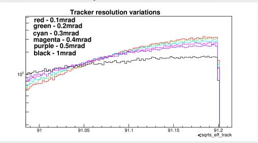
One should stick to the foreseen 0.1 mrad muon angular resolution (100  $\mu$ m track resolution for TPC) to be known with 0.1 mrad margin
