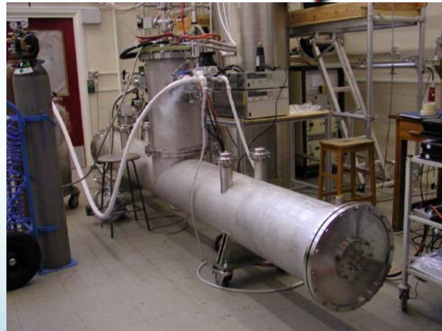
SC undulator prototype developed at RAL
