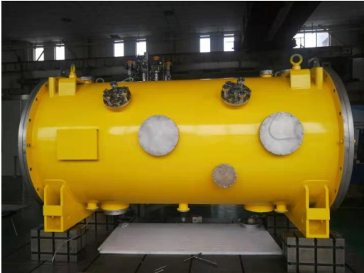
Cryomodule vacuum vessel and cold mass
