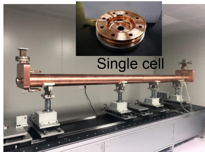
The accelerating structure under tuning
