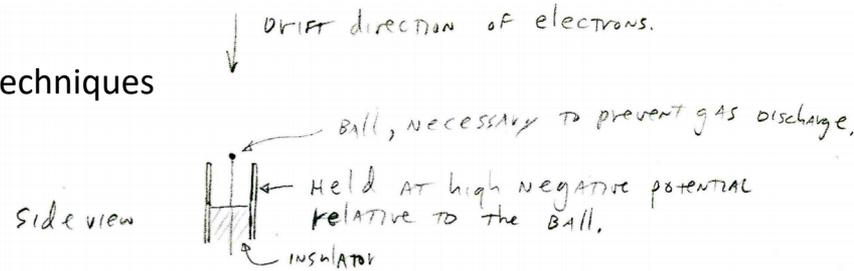
Fig. 4 Ball-wire detector (For honey comb)
