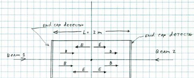
Fig 1b. colliding beam geometry, using thin foil in plane  $z=0$  to establish a symmetric ELECTRIC FIELD.
