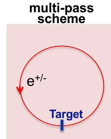
Add a single target in a low- $\beta$  and dispersion-free location (Interaction Point)
