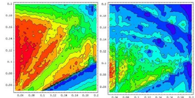
Beam-beam simulations showing that synchrotron resonances are suppressed
