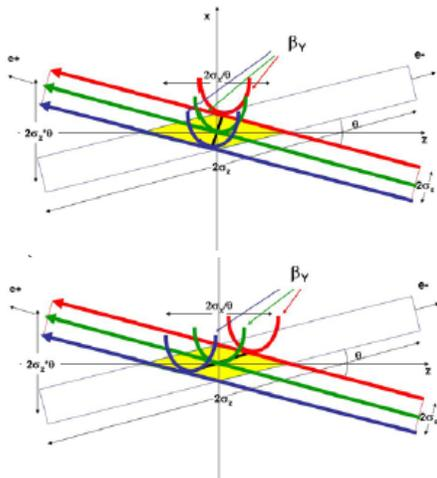
Placed at a proper phase advance they produce a constant  $\beta_y$  along the longer axis of the overlap area, thus suppressing the hourglass effect, enhancing luminosity.
