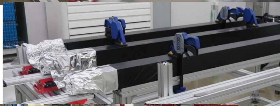
Closeup view of the interface between scintillator & lightguide
