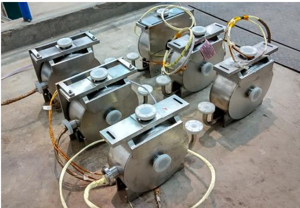
ADS linac, 5T SC solenoids 26 sets completed
