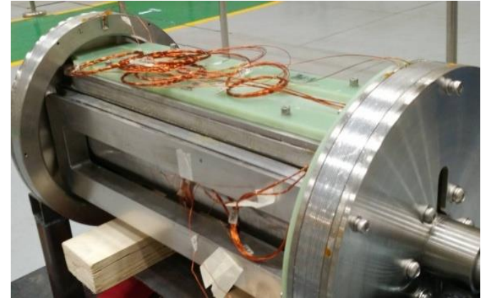
US FRIB, 8-9T superconducting solenoids 80 sets completed
