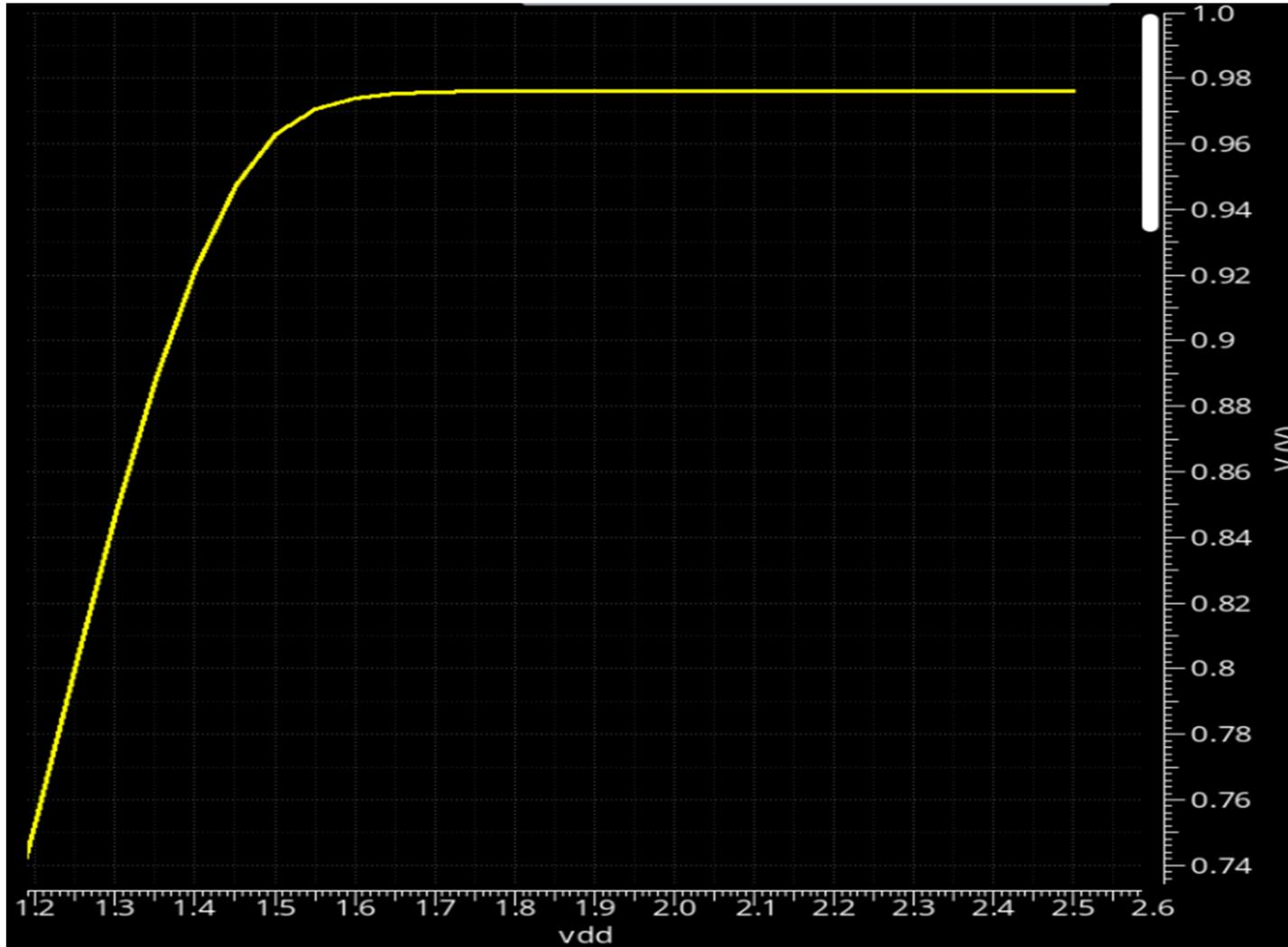
$V_{bg}=0.976 \text{ V @ } V_{dd} \geq 1.8 \text{ V}$
